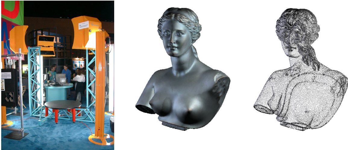
Figure 7.19: 3D scanners (left) produce large point clouds (right) from real objects (middle).
